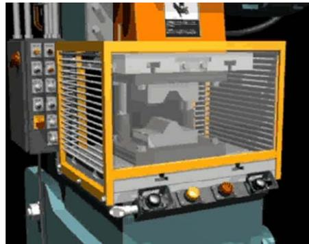
Figure 1. Power press with a fixed barrier guard [13]
